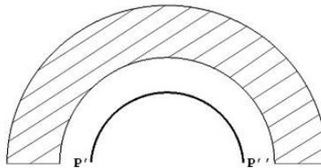
**Fig. 1** Cross section of the unimodal PVDF transducer that can operate alternatively as transmitter or receiver. The  $\lambda/4$  back reflector is also shown
