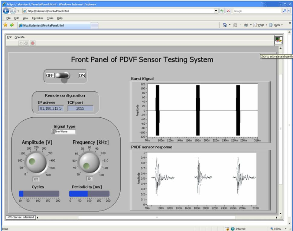
Fig. 7. HTML page with System’s Front Panel
