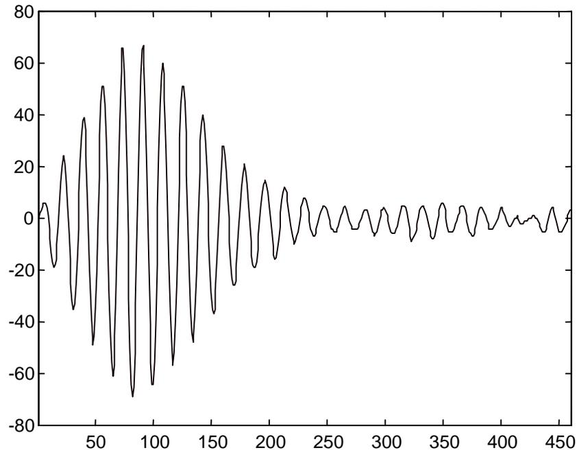
**Fig. 3.** Typical signal received by the transducer in the pulse-echo mode. The transmitter was excited by a high voltage Dirac like pulse generated by a Panametrics 5058 PR
