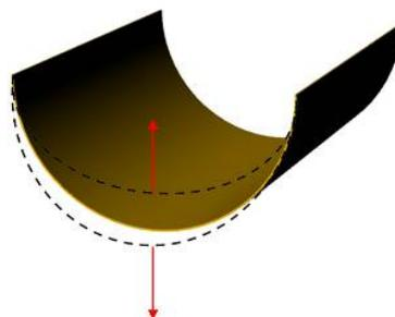
**Fig. 2.** Particular arrangement and radial vibration mode of the piezoelectric sheet
