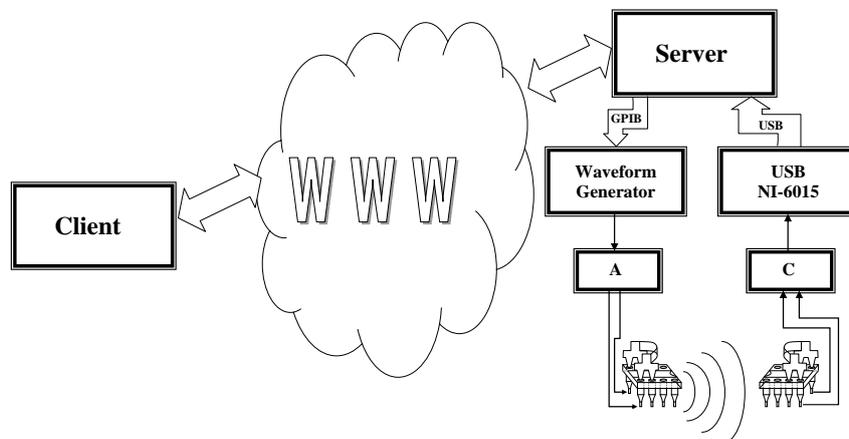
**Fig. 5.** Web System's Architecture
