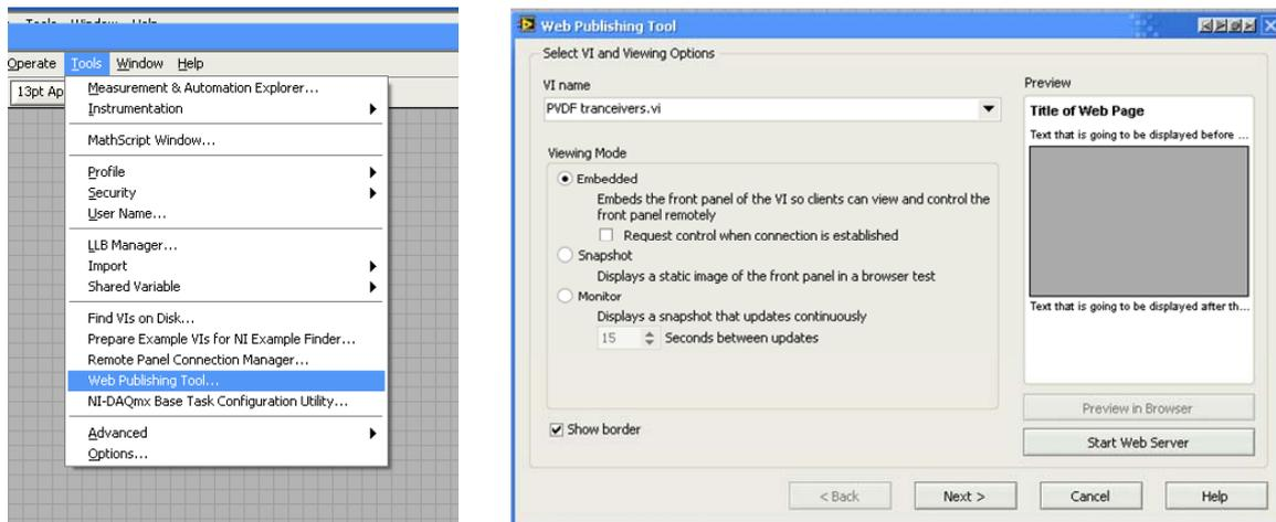
**Fig. 4.** Web Publishing Tool command and its configuration window
