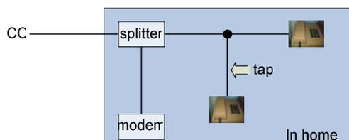
Figure 1: good positioning of the splitter
