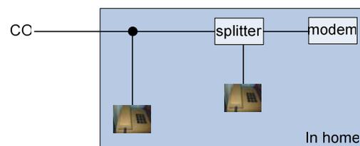
Figure 2: bad positioning of the splitter
