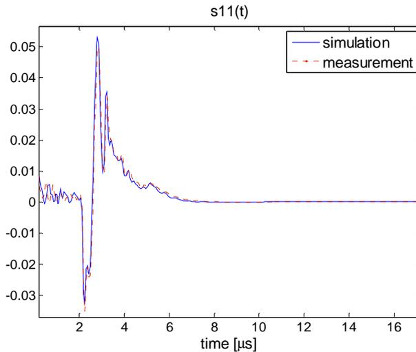
Figure 4. The comparison measurement-simulation for L(LTL)L topology
