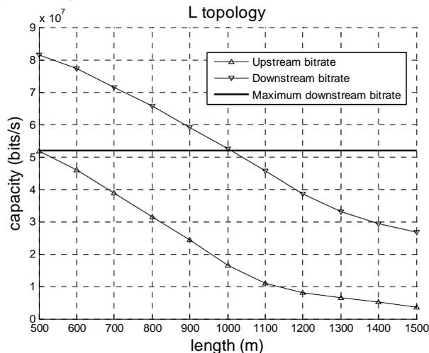
Figure 5. The influence of the length on the capacity
