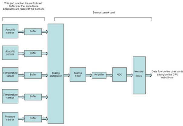
Fig. 4 Block diagram of sensor board
