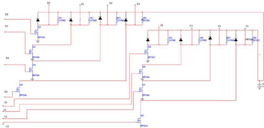
Fig. 9 Electric circuit for controlling two stepper motors
