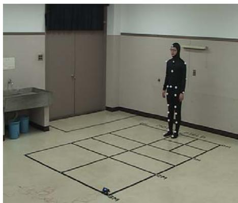
Fig. 2 measurement of human walking motion
