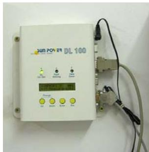
Fig.3 – Data Logger Sun Power DL100
