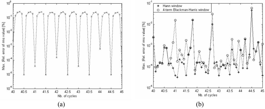
Fig. 3. The maximum of the relative errors modulus of the rms value as function of the recorded cycles number obtained during  $\varphi$  scan in the range  $[0, 2\pi)$ rad. The rms value is estimated by: a)  $\hat{X}_{rms}$  ('x' mark and dotted line) and b)  $\tilde{X}_{rms}$  with Hann window (star and dotted line) and 4-term Blackman-Harris (circle and dotted line).
