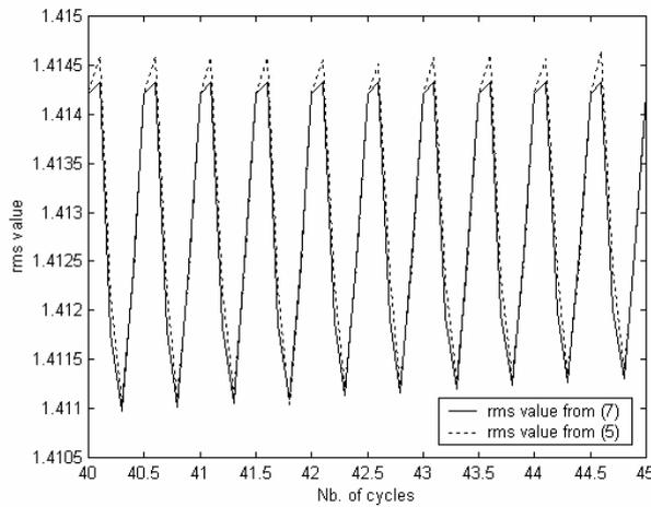
Fig. 1.  $X_{rms}$  (solid line) and  $\hat{X}_{rms}$  (dotted line) as a function of the number of recorded cycles.
