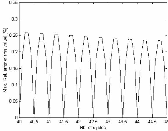
Fig. 2. The maximum of the relative error modulus of the rms value measurement as function of the number of recorded cycles obtained during  $\varphi$  scan in the range  $[0, 2\pi]$  rad.
