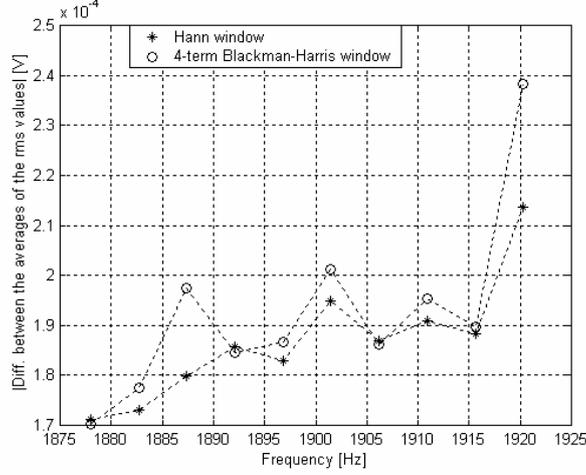
Fig. 4. The modulus of the difference between the average of the sinewave rms values estimated by the proposed method and the one of the rms values estimated by means of the IpDFT method as a function of frequency. In the proposed method the Hann window (star and dotted line) and the 4-term Blackman-Harris window (circle and dotted line) are used.
