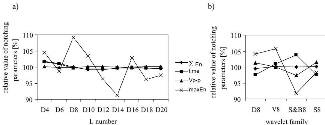
Fig. 5. Relative values of notching analysis; a) different filter lengths of Daubechies filters, b) different wavelets families
