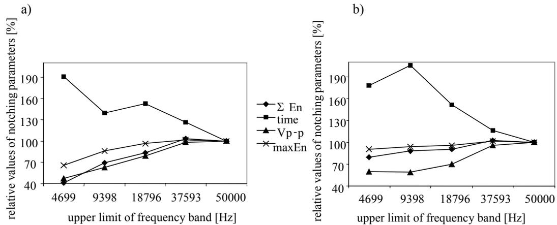
Fig. 4. Relative values of notching analysis for both cases: a) shaft generator and two diesel generators working in parallel, b) shaft generator working alone
