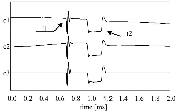
Fig. 2. Example of notching analysis; curve  $c_1$  – original voltage samples, curve  $c_2$  – voltage components of 587 – 50000 Hz frequency band, curve  $c_3$  – filtered two impulses  $i_1$  and  $i_2$  by means of formula (3)
