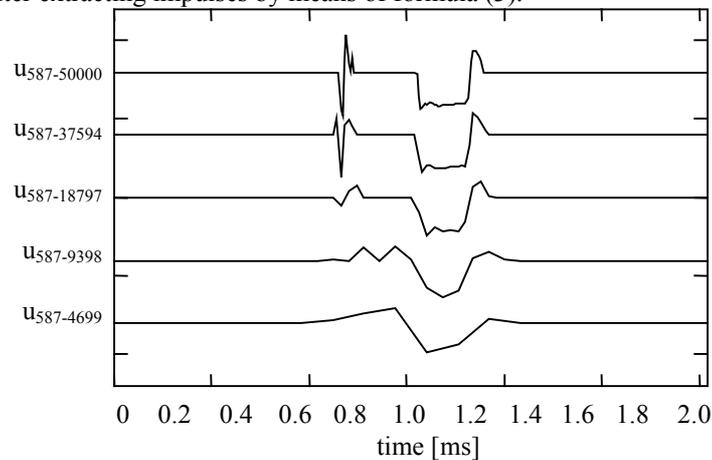
Fig. 3. Reconstructed higher frequency components for five different frequency bands (represented as subscripts in figure designations) and respectively decimated samples
