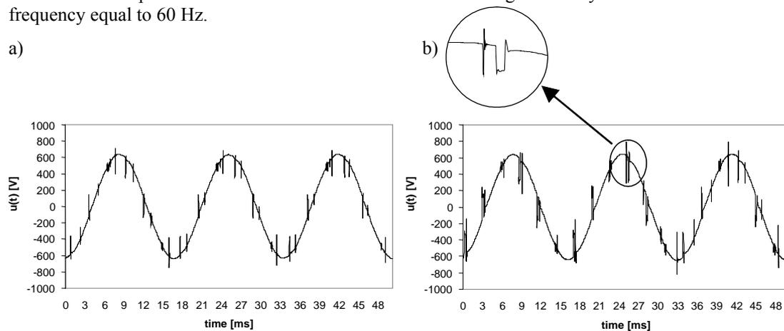
Fig. 1. Exemplary voltage in isolated electric power system: a) shaft generator and two diesel generators working in parallel, b) shaft generator working alone
