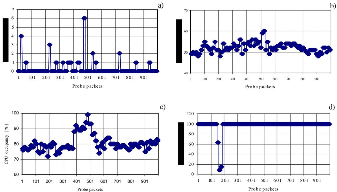
Figure 6 CPU occupancy measurement on 1000 probe packets: a) low occupancy, b) about 50% of occupancy, c) about 80% of occupancy, and d) full occupancy.
