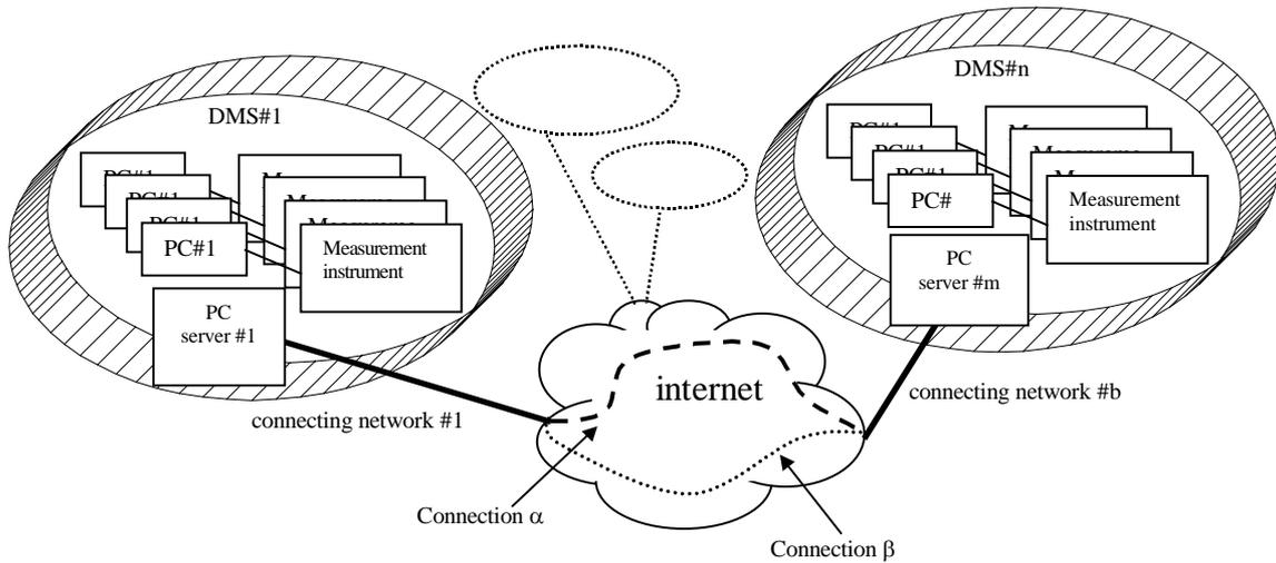
Figure 1 General architecture of the DML.
