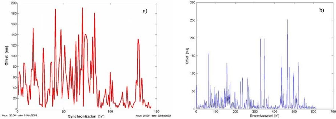
Figure 3 PC synchronization in presence of random perturbation a) every ten minutes, and b) every one minute.
