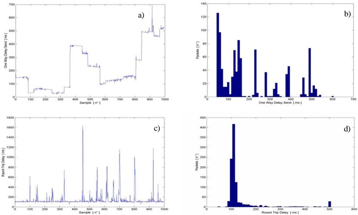
Figure 5 a), and c), OWD and RTD measurement executed on the WAN2 for each probe packet, and b), and d) the corresponding occurrences of the time delays.
