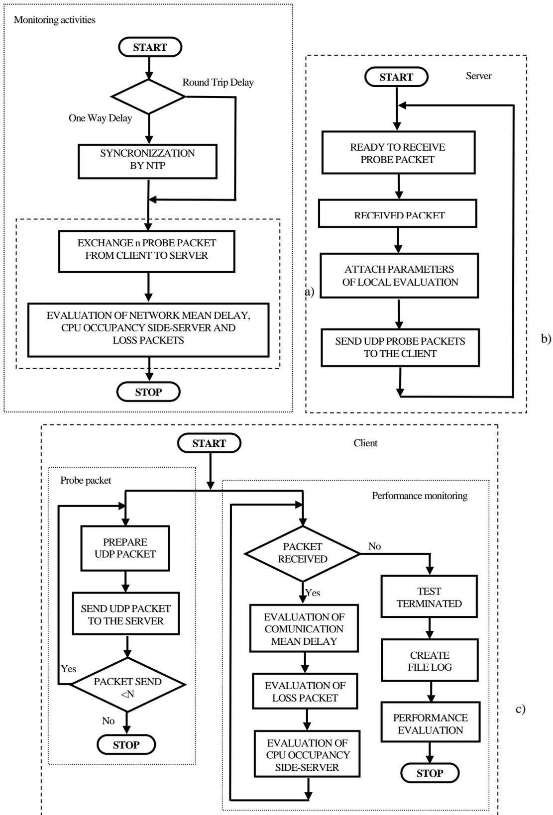
Figure 2 Flow diagram implementing the propose method.
