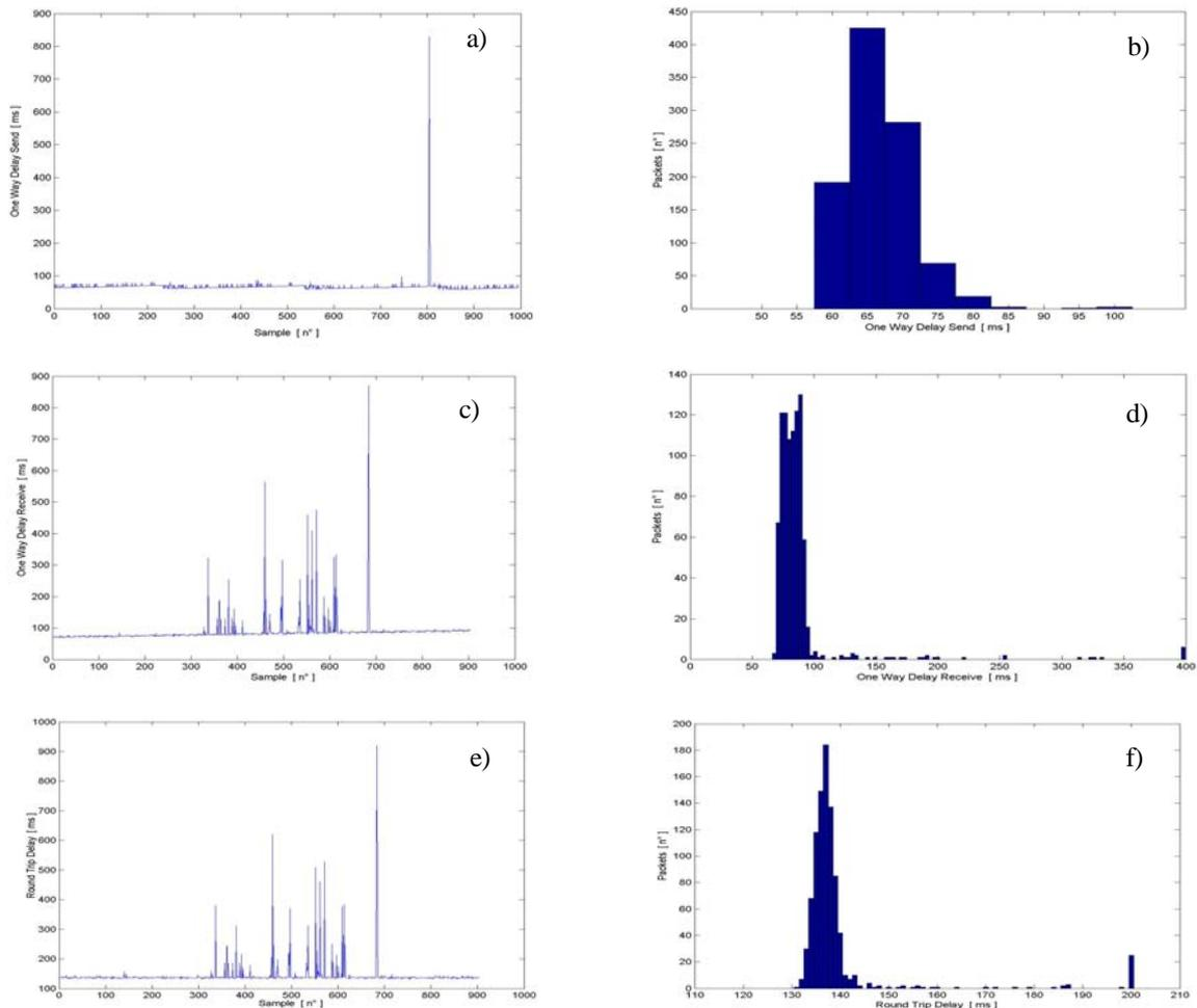
Figure 4 a), c), and e) OWD and RTD measurement executed on the WAN1 for each probe packet, and b), d), and f) the corresponding occurrences of the time delays.
