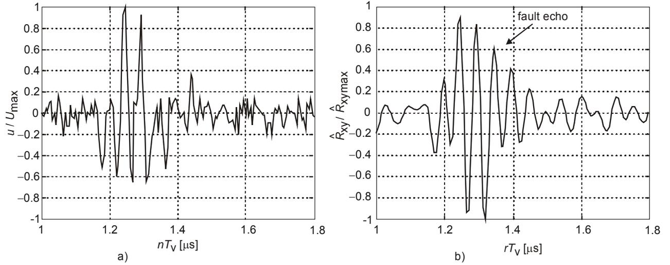
Fig. 3 Detail of ultrasonic signal on special gauge and signal de-noising (a – raw signal, b – correlation filtered signal)
