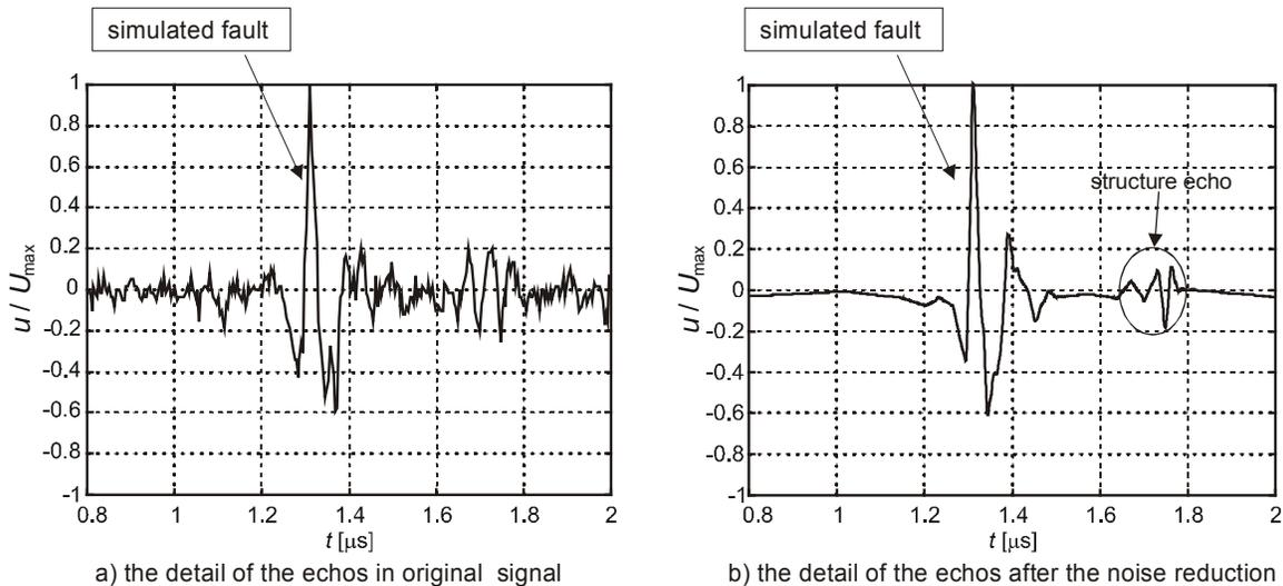
Fig. 2: Detail of ultrasonic signal on special gauge and signal de-noising (*SNRE*  $\approx$  54 dB).
