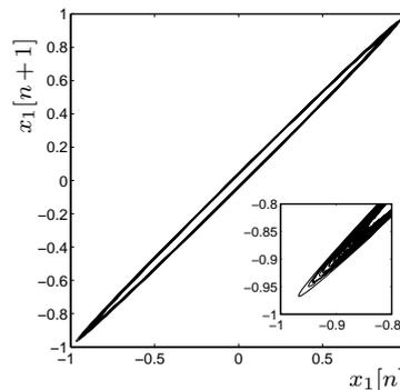
Fig. 4. Trajectory of the  $x_1[\cdot]$  state variable on the phase plane. In the inset, a zoomed portion of such a trajectory is shown. Since the orbits are not superimposed, the corresponding waveform is not exactly periodic.
