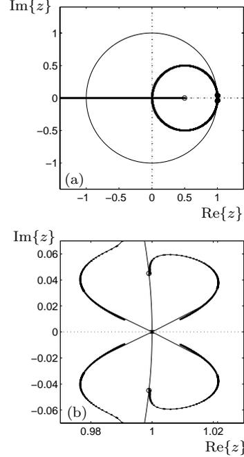
Fig. 6. Root locus of the resonator-modulator equivalent circuit when the generated sinusoid has a 22 kHz frequency. In (a) the full root locus is shown, while in (b) a zoomed portion of (a) is plotted around  $z = (1, 0)$ .
