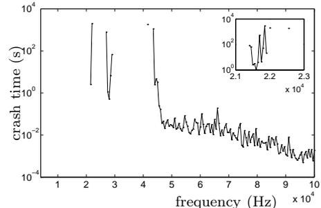
Fig. 3. Crash time of the oscillator as a function of the frequency. As  $a_{12}a_{21}$  increases, the stability of the oscillator deteriorates.
