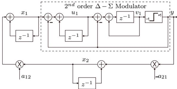
Fig. 1. Block diagram of the considered modulator–resonator. The parameters  $a_{12}$  and  $a_{21}$  determine the frequency of the generated sinusoid.
