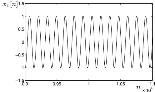
Fig. 8. Time waveform of  $x_1[\cdot]$  at a frequency of 22 kHz. Due to the insertion of soft limiters, the waveform does not diverge after 20 minutes.
