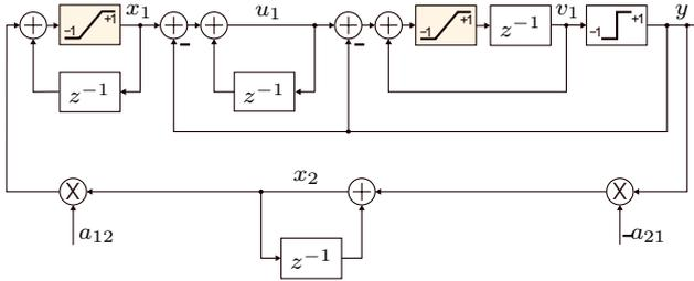
Fig. 7. Block diagram of the modified  $\Delta$ - $\Sigma$  modulator-resonator. Circuit stabilization is achieved through the 2 soft limiters highlighted in grey.
