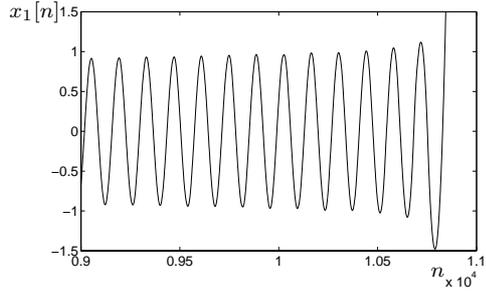
Fig. 2. Time waveform of  $x_1[\cdot]$ . The signal frequency is 22 kHz and the waveform diverges after about 20 real–time minutes.
