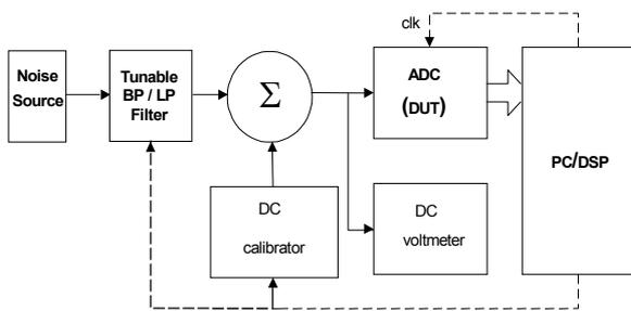
Fig. 2 Arrangement of testing system for ADC stochastic testing
