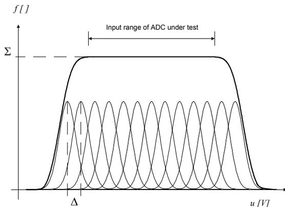
Fig.1 Stochastic test signal generation
