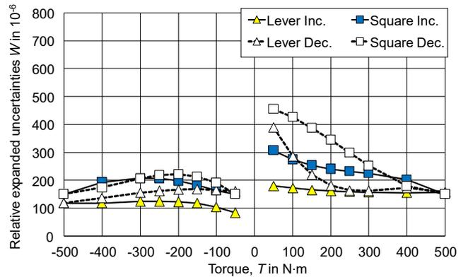
Figure 17. Relative expanded uncertainties of calibration for TS500
