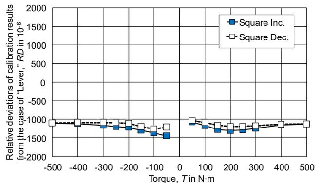
**Figure 13.** Relative deviations of calibration results from the case of changing lever direction, for TS500.
