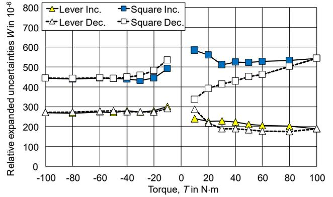
Figure 16. Relative expanded uncertainties of calibration for TTS/100Nm
