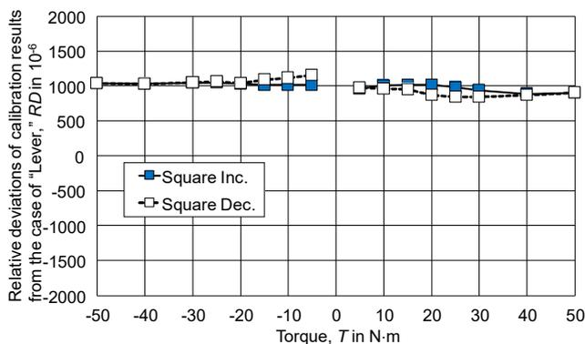
**Figure 11.** Relative deviations of calibration results from the case of changing lever direction, for TS50.
