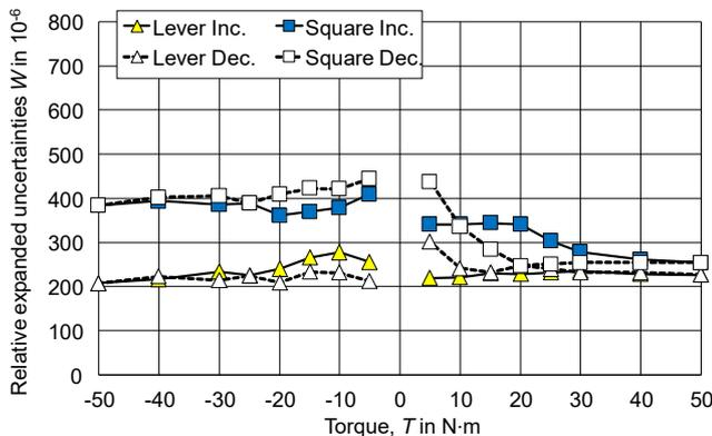
Figure 15. Relative expanded uncertainties of calibration for TS50
