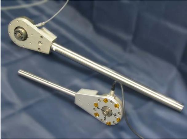
**Figure 5.** A photograph of transducers TS50 (lower side) and TTS/100Nm (upper side).
