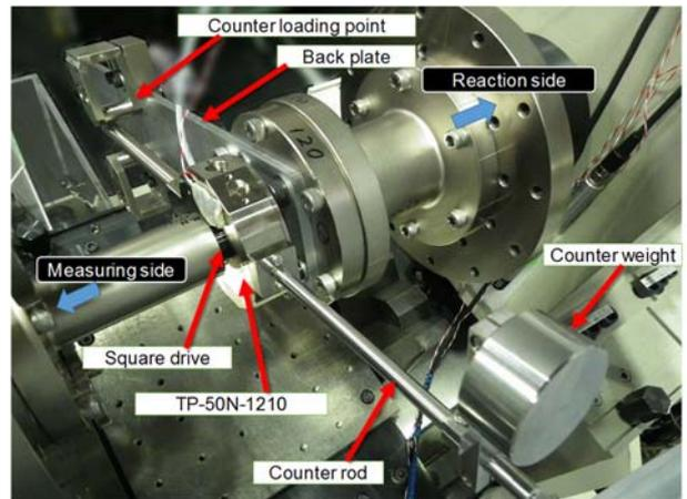
**Figure 8.** An example of installation of transducer on the 1-kN·m-DWTSM by “Lever” way (TP-50N-1210, at the mounting position of 0 degree for the case of counterclockwise torque).
