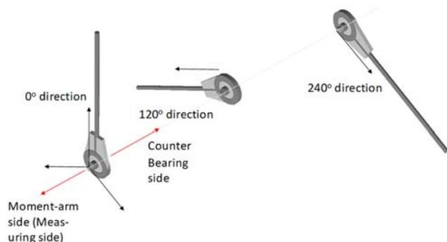
Figure 2. Rotational mounting position change by changing lever direction ("Lever" way).
