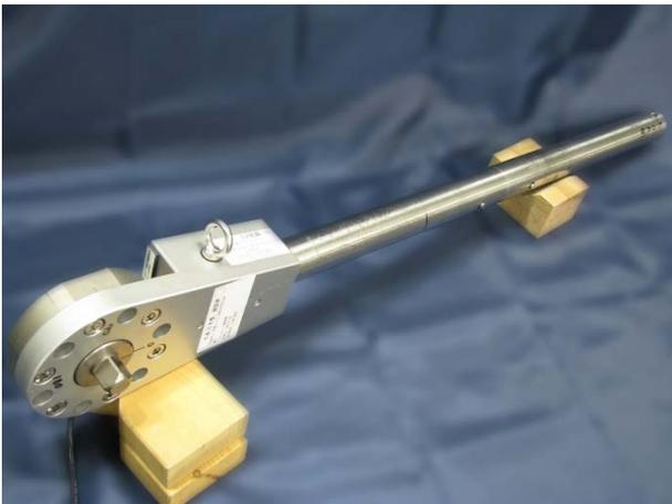
**Figure 6.** A photograph of transducer TS500.
