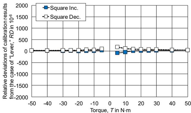
**Figure 10.** Relative deviations of calibration results from the case of changing lever direction, for TP-50N-1210.
