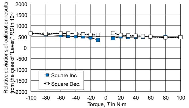
**Figure 12.** Relative deviations of calibration results from the case of changing lever direction, for TTS/100Nm.
