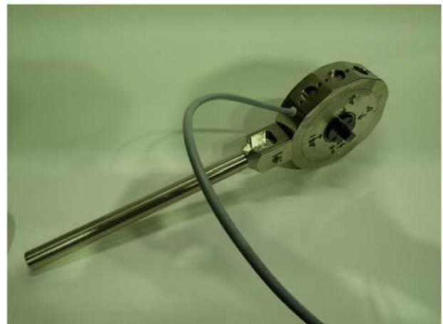
**Figure 4.** A photograph of transducer TP-50N-1210.
