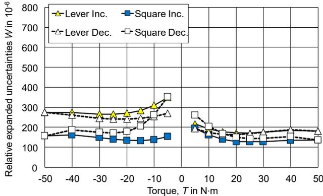
Figure 14. Relative expanded uncertainties of calibration for TP-50N-1210
