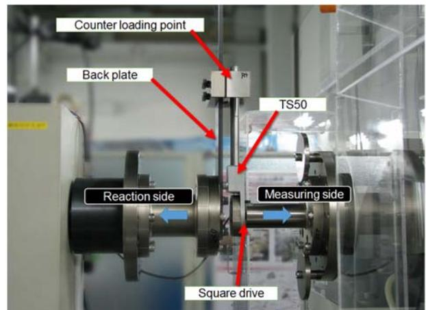
**Figure 9.** An example of installation of transducer on the 1-kN·m-DWTSM by “Square” way (TS50, at the mounting position of 0 degree for the case of clockwise torque).
