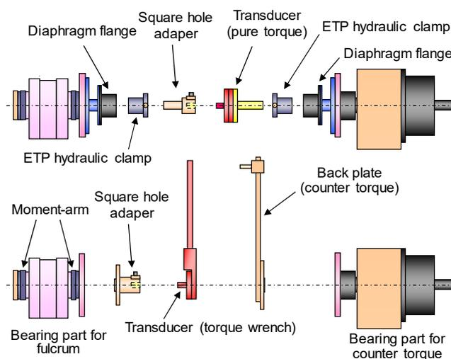
Figure 1. Setup of transducer on the TSM.
