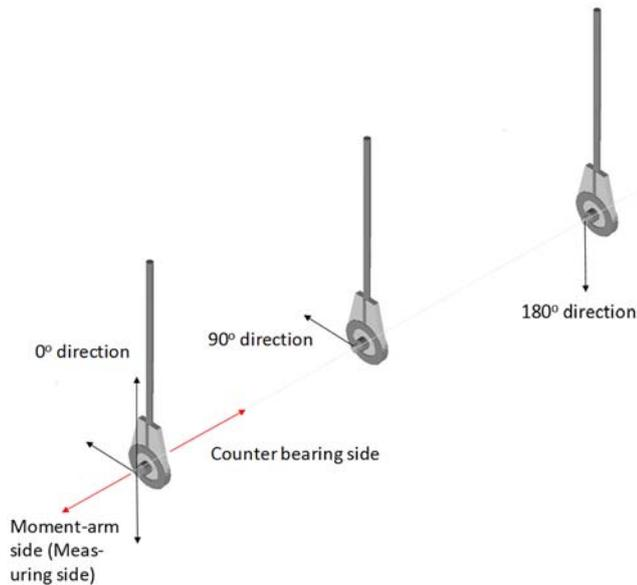
**Figure 3.** Rotational mounting position change by changing detachable square drive (“Square” way).
