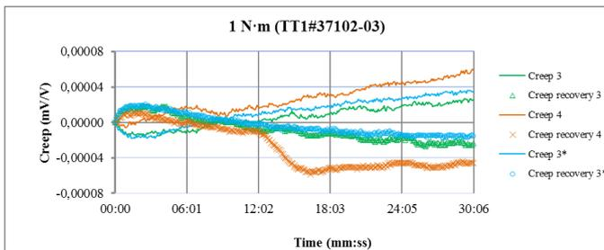
**Figure 9: Effect of humidity on the creep of a 1 N·m torque transducer**
