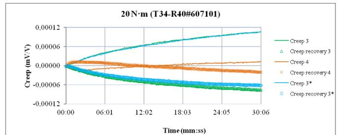
**Figure 13: Effect of humidity on the creep of a 20 N·m torque transducer**
