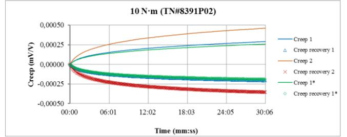
**Figure 6: Effect of temperature on the creep of a 10 N·m torque transducer**
