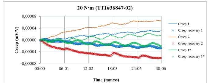
**Figure 7: Effect of temperature on the creep of 20 N·m torque transducer**
