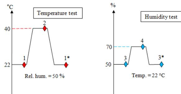
**Figure 1: Environmental test sequence for (a) temperature (left) and (b) relative humidity (right)**
