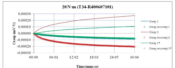
**Figure 8: Effect of temperature on the creep of 20 N·m torque transducer**
