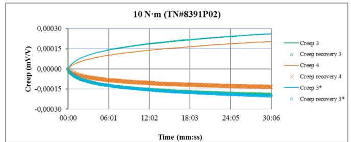
**Figure 11: Effect of humidity on the creep of a 10 N·m torque transducer**
