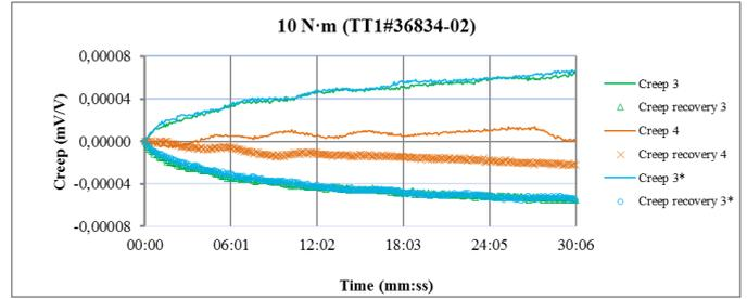
**Figure 10: Effect of humidity on the creep of a 10 N·m torque transducer**
