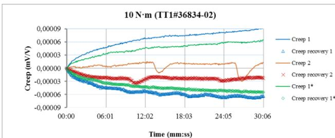
**Figure 5: Effect of temperature on the creep of a 10 N·m torque transducer**
