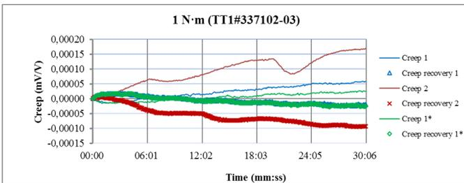
**Figure 4: Effect of temperature on the creep of a 1 N·m torque transducer**
