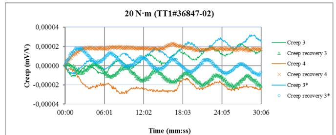
**Figure 12: Effect of humidity on the creep of a 20 N·m torque transducer**
