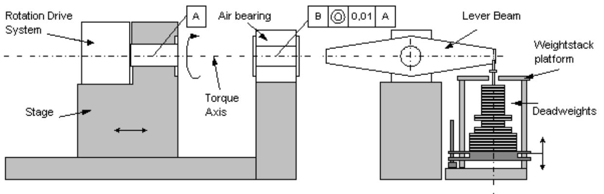
Figure 2. Principal components of the LNE 50 Nm deadweight torque standard machine
