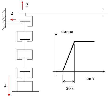
Figure 11. Principle of weightstack platform retractable end stops
