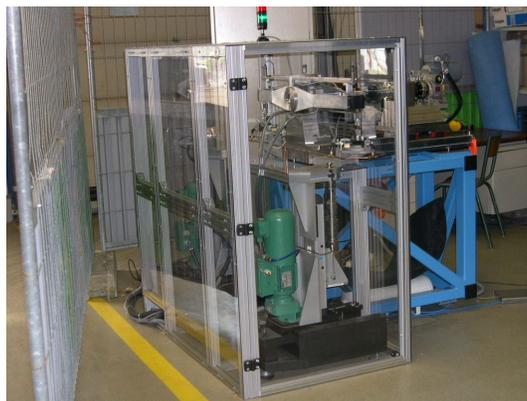
Figure 1. The new LNE 50 Nm deadweight torque standard machine
