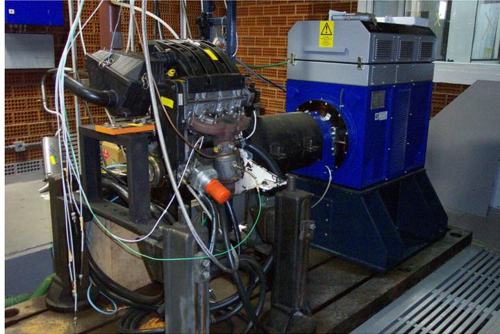
Figure 02 – Engine test bench of Lamoc/Inmetro (in line torque transducer mounted inside)
