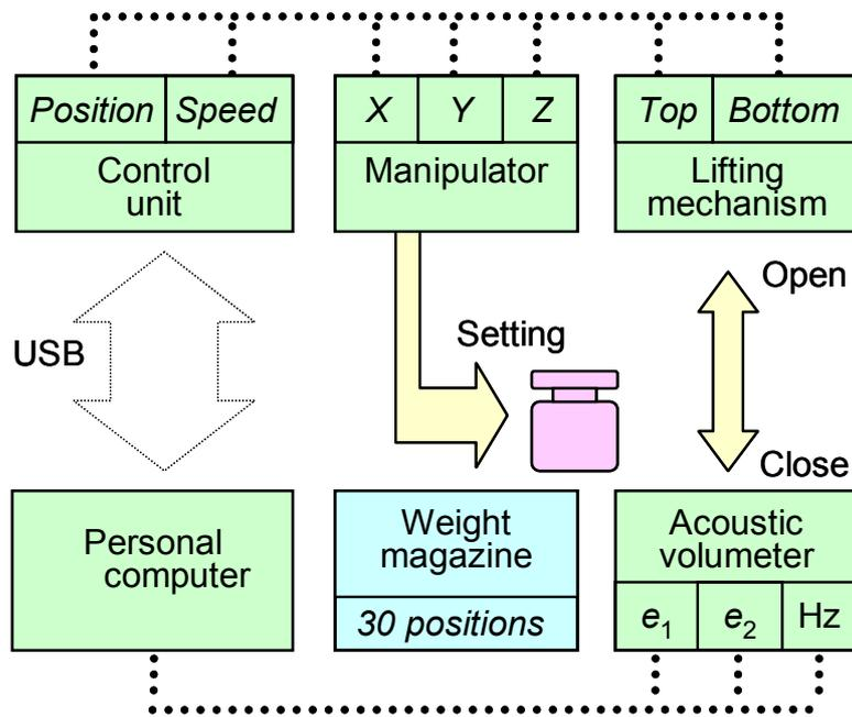
Figure 2 Block diagram of the automated system
