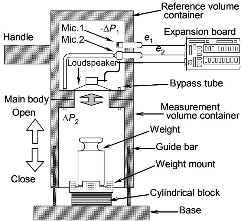
Figure 1 Schematic drawing of the acoustic volumeter
