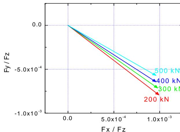
**Figure 5** : Side force components of the 500 kN deadweight force machine
