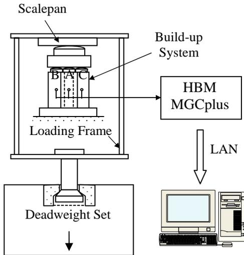
**Figure 3** : Experimental set-up for side force components
