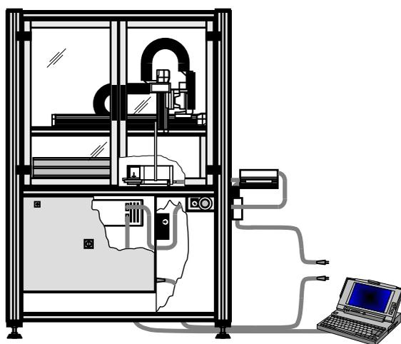
**Figure 2.** Schematic drawing of the automatic comparator, which consists of a cabinet containing a weight magazine, a robot, a comparator balance, and a control unit. The equipment is operated by a PC
