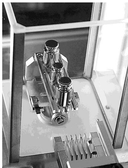
**Figure 5.** The weight receiver of the a100 comparator.
