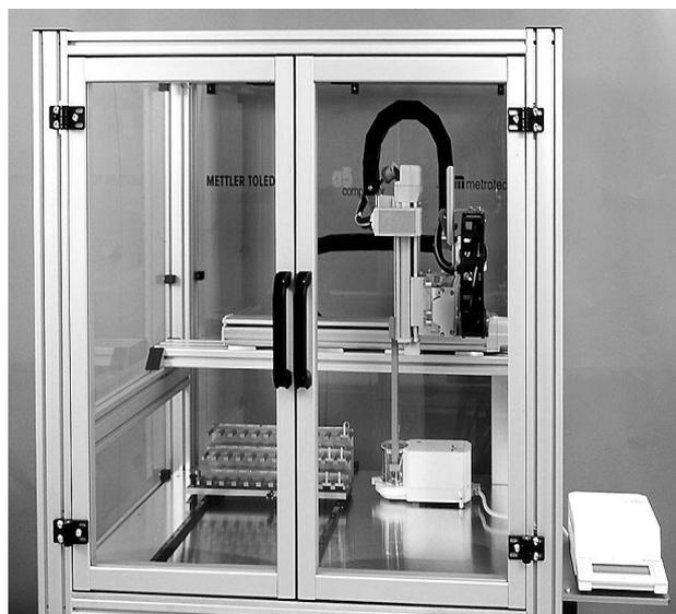
**Figure 6.** Upper front view of the a5 automatic comparator.
