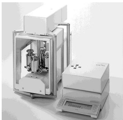
**Figure 1.** An example of a 1kg mass comparator with a four places turntable
