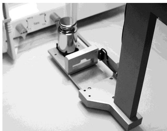
**Figure 4.** A weight loaded on its weight carrier is being moved from the magazine to the balance's weight receiver.
