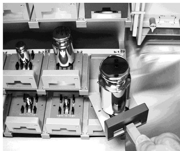
**Figure 3.** The weight magazine of the a1000comparator
