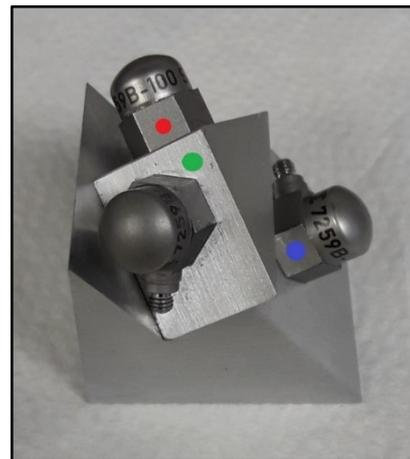
Figure 6: Pseudo tri-axial accelerometer
