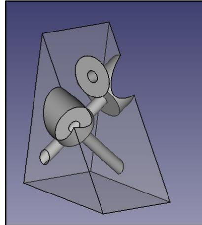
Figure 5: Wedge design for embedded tri-axial accelerometers
