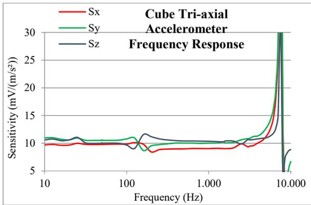
Figure 3: Cube tri-axial accelerometer frequency response
