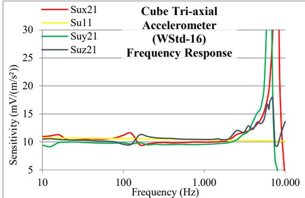
Figure 4: WStd-16 frequency response, mounted in x, y, and z axis positions and the single axis primary calibration result ( $S_{u11}$ )
