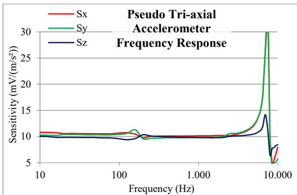
Figure 7: Pseudo tri-axial accelerometer frequency response
