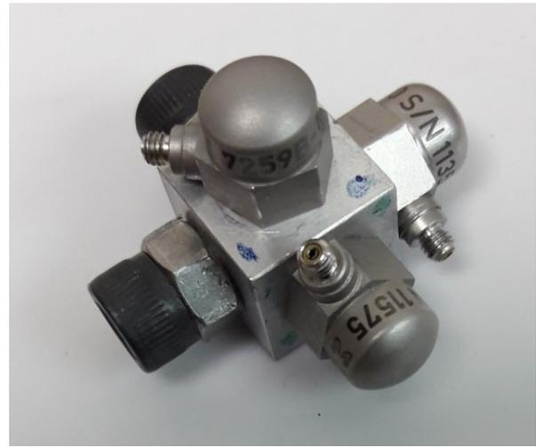
Figure 2: Cube tri-axial accelerometer showing the  $10 \text{ mm}^3$  aluminium block, three ENDEVCO accelerometers and two M5 allen screw/nut counterweights
