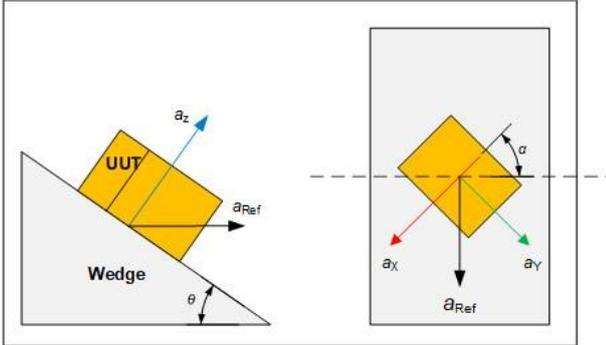
Figure 1: Inclined clamp (wedge) configuration
