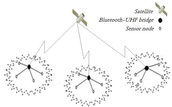
Fig. 8. Sensors network architecture
