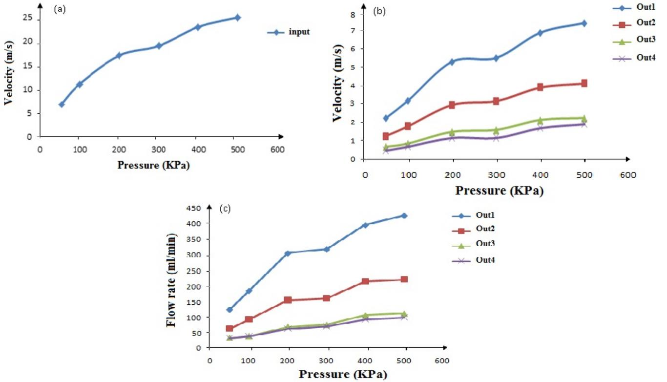
Fig. 2. (a) Velocity at the inlet (b) Velocity at the outlets (c) Flow rate at the outlets
