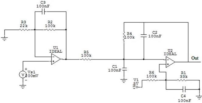
Fig. 4. pH probe circuit sensing
