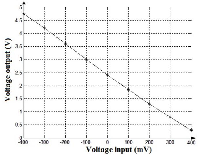
Fig. 5. Characteristic curve of pH probe circuit sensing
