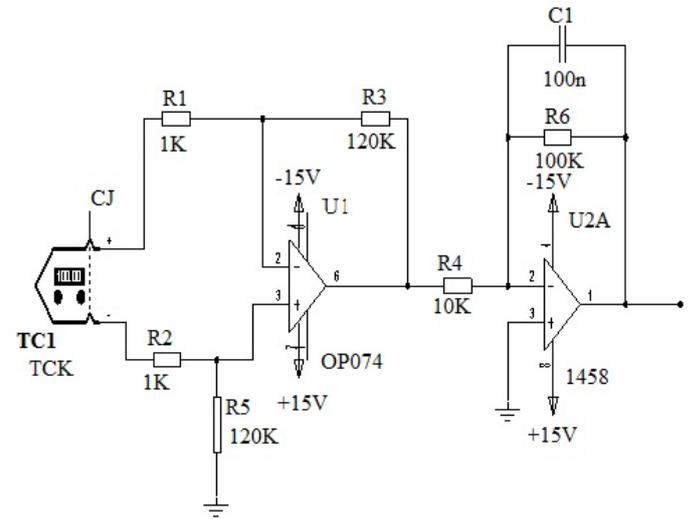
Fig. 6. Temperature interfacing circuit
