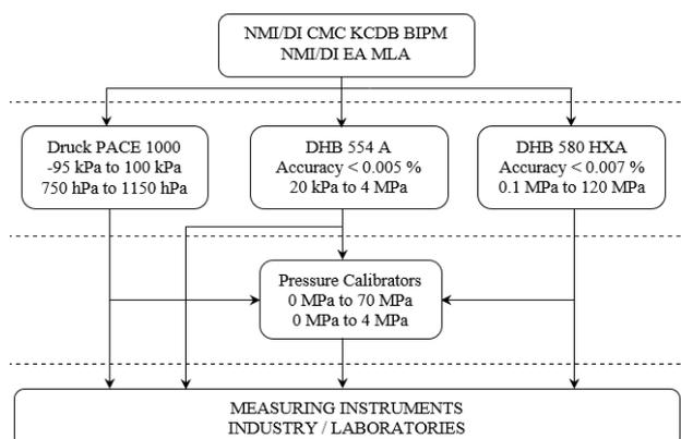
Figure 3: Traceability scheme for the Laboratory for Pressure
