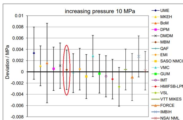
Figure 4: Deviations from the reference value with uncertainties at 10 MPa in the EURAMET.M.P-S13 interlaboratory comparison [5]
