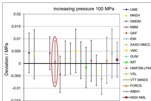
Figure 5: Deviations from the reference value with uncertainties at 100 MPa in the EURAMET.M.P-S13 interlaboratory comparison [5]
