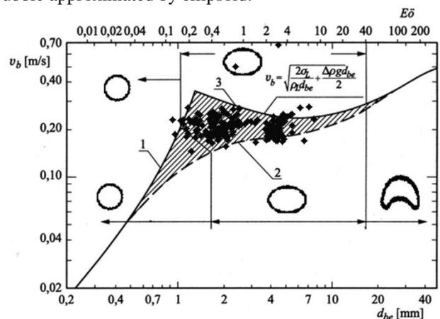
Fig.12. Movement rate of the gas bubbles depending on their diameters [13].
