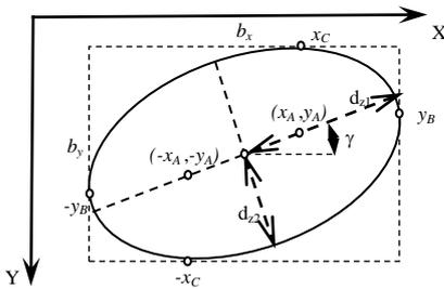
Fig. 6: Ellipsoide projection into  $XY$  plane
