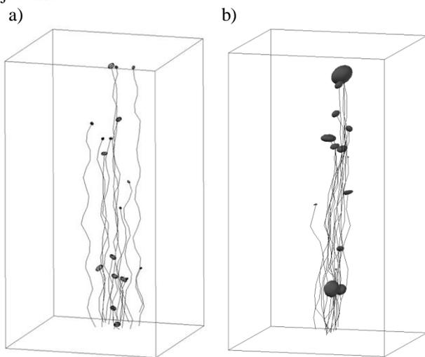
Fig. 8: Reconstruction of the bubble movement trajectory for gas streams a) 0.001 m<sup>3</sup>/h b) 0.02 m<sup>3</sup>/h
