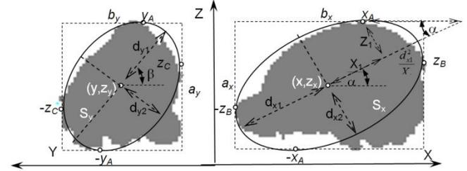
Fig. 4: View of the bubble image after binary conversion
