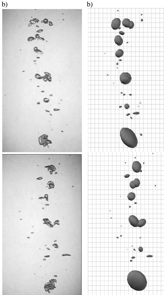
Fig.10. Flow images for gas streams 0.06 m<sup>3</sup>/h image from the camera a) image from the tomograph. b)
