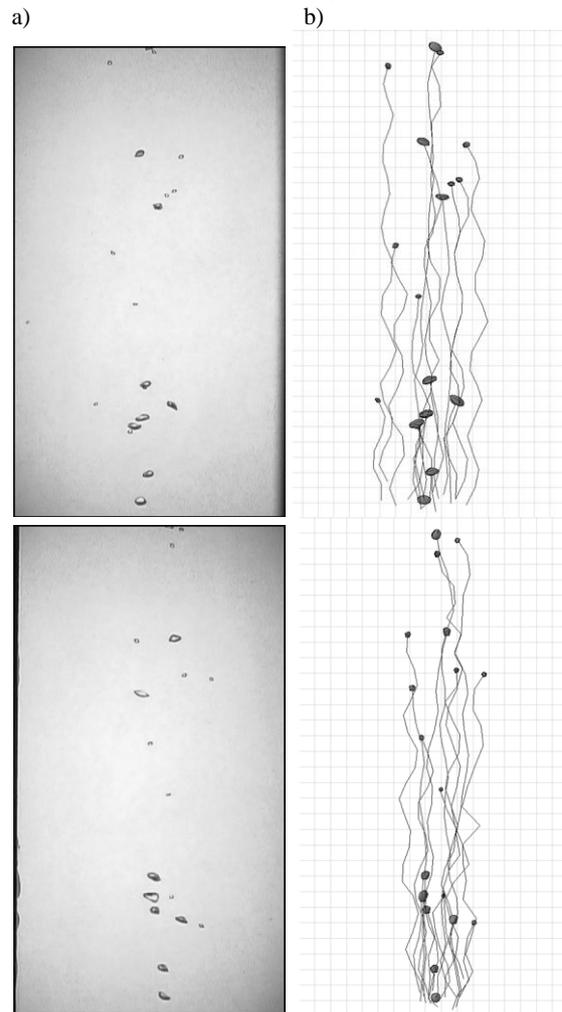
Fig.9. Flow images for gas streams 0.001 m<sup>3</sup>/h a) image from the camera, b) image from the tomograph.
