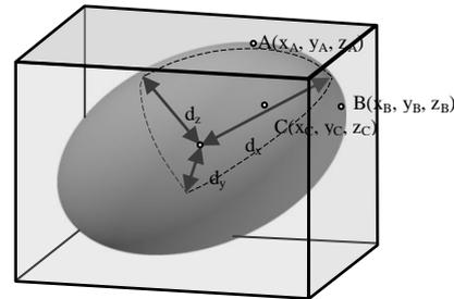
Fig. 5: Approximation of the bubble shape with ellipsoid.
