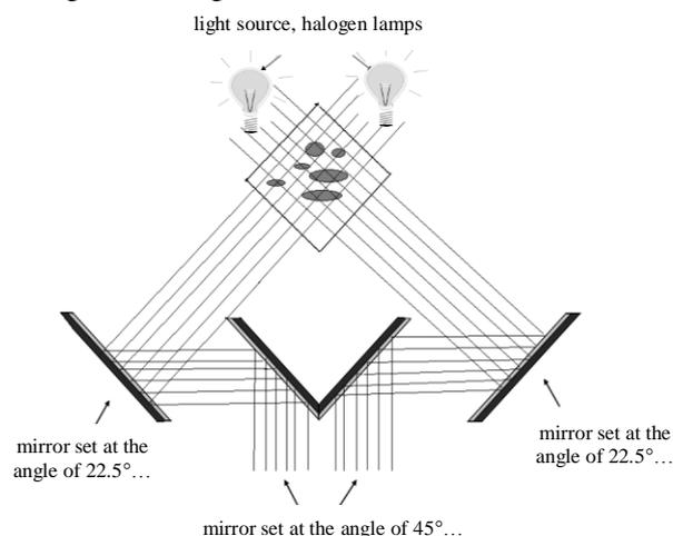
Fig. 1: Principle of image tomograph operation.
