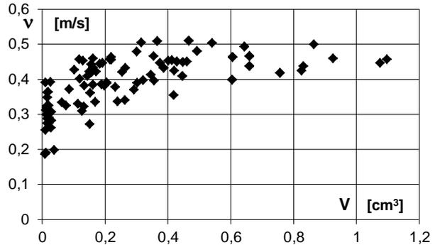
Fig.11. Dependence of the bubble movement rate and the bubble volume
