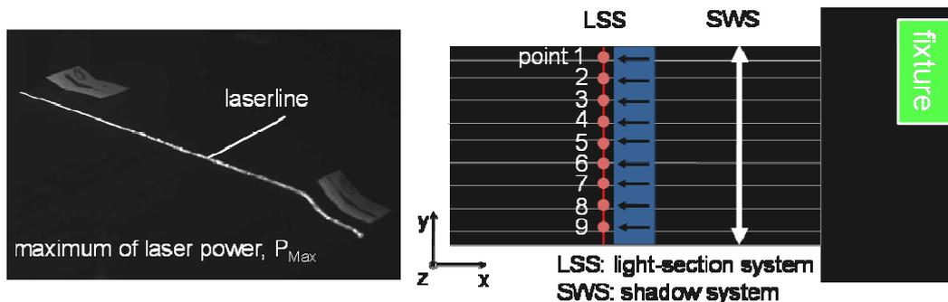
Fig.2: Measurement configuration: left: contrast of the laser line, right: measuring points
