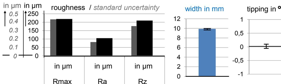
Fig. 4: Left: roughness results, middle: width measurement, right: tipping of the fiber tape
