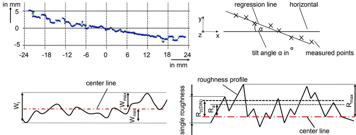
Fig. 3: Left upper: measured contour with basic form, right upper: principle of tilt measurement, bottom left: ripple, bottom right: roughness
