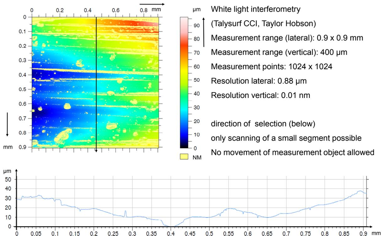
Fig. 5: Measurement with WLI: upper: colour results, bottom: selected area, scanning height
