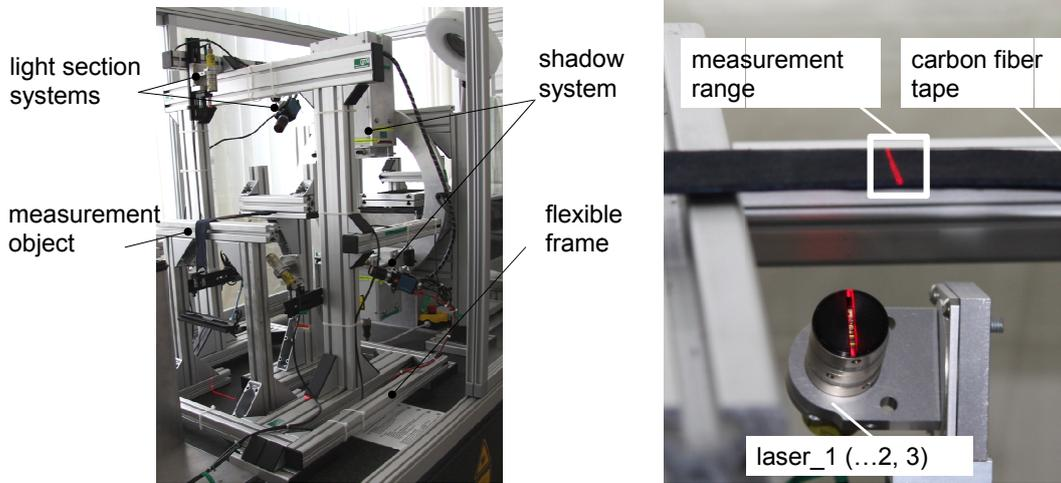
Fig. 1: Optical bi-sensor measurement prototype, left: isometric view, right: carbon-fiber tape
