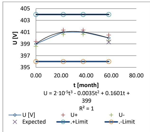
Figure 2: The calibration history and expected value in a single point of voltage measurement range
