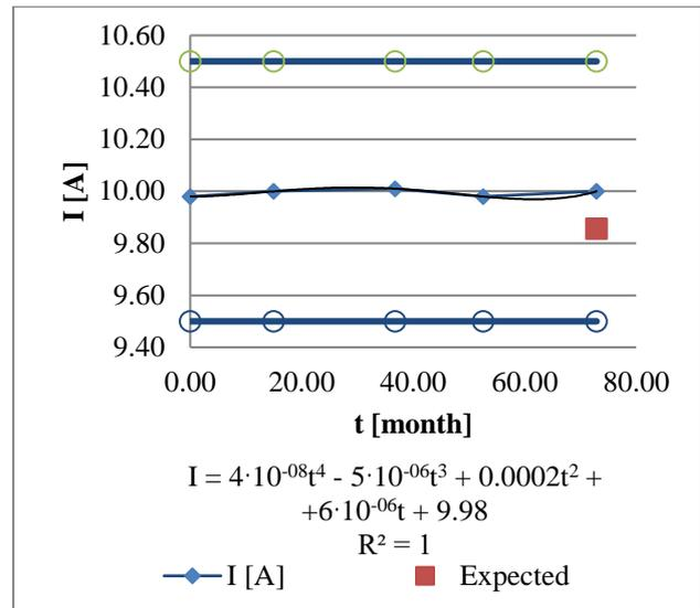
Figure 1: The calibration history and expected value in a single point of current measurement range
