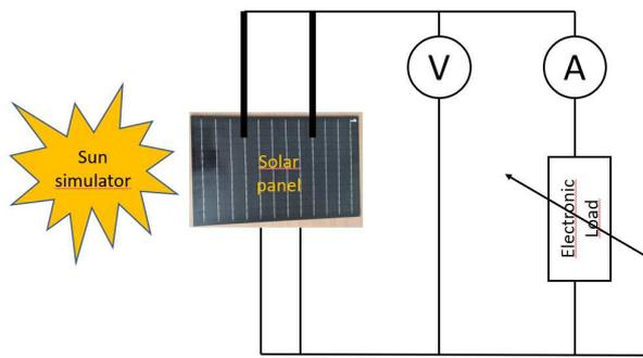
Figure 4: Operating principle of the solar simulation test
