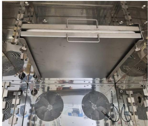
Figure 2: Opening on top of the climatic chamber – with sealing
