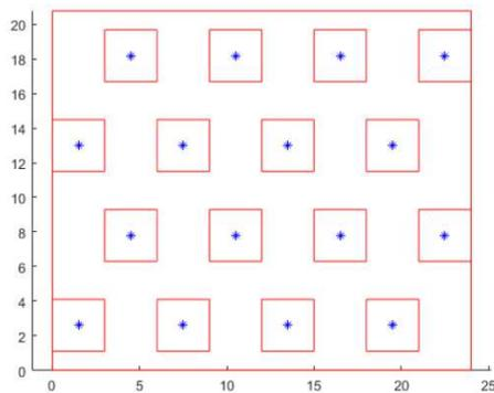
Figure 5: Solar simulator – a possible arrangement of LEDs [units in cm] (15.05.2022 University of Pannonia, Faculty of Engineering, Department of Process Engineering)
