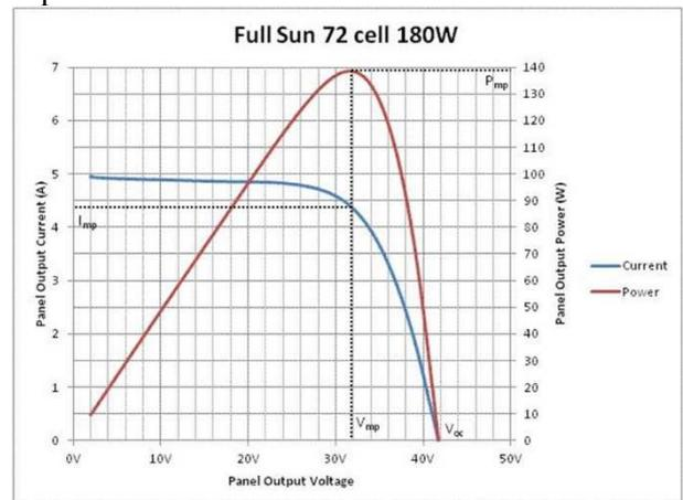
Figure 3: [2] Trevor Barcelo, Solar panel I-V curve showing maximum power
