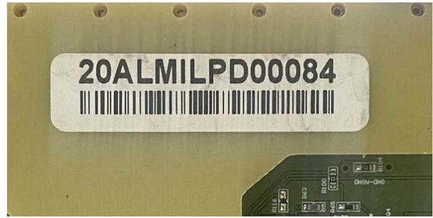
Figure 4: Label example on a PDB. Any PDB has a barcode that is a unique code.
