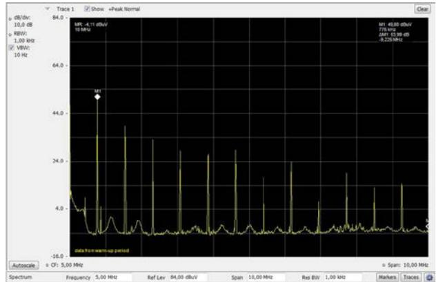
Figure 6: Noise spectrum of LTM4913 with 2.5 output voltage
