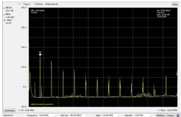
Figure 7: Noise spectrum of LHC4619 with 2.5 output voltage
