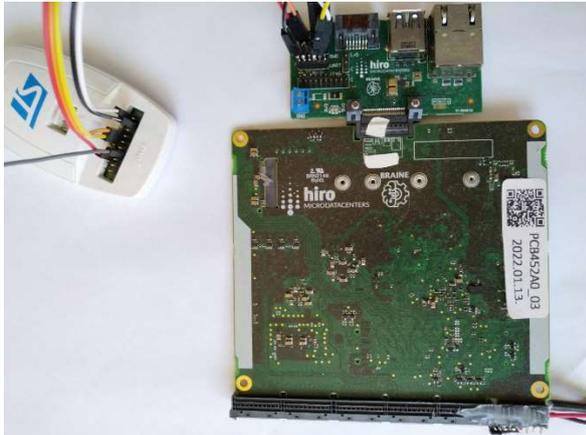
Fig. 4. Manufactured CPU Node
