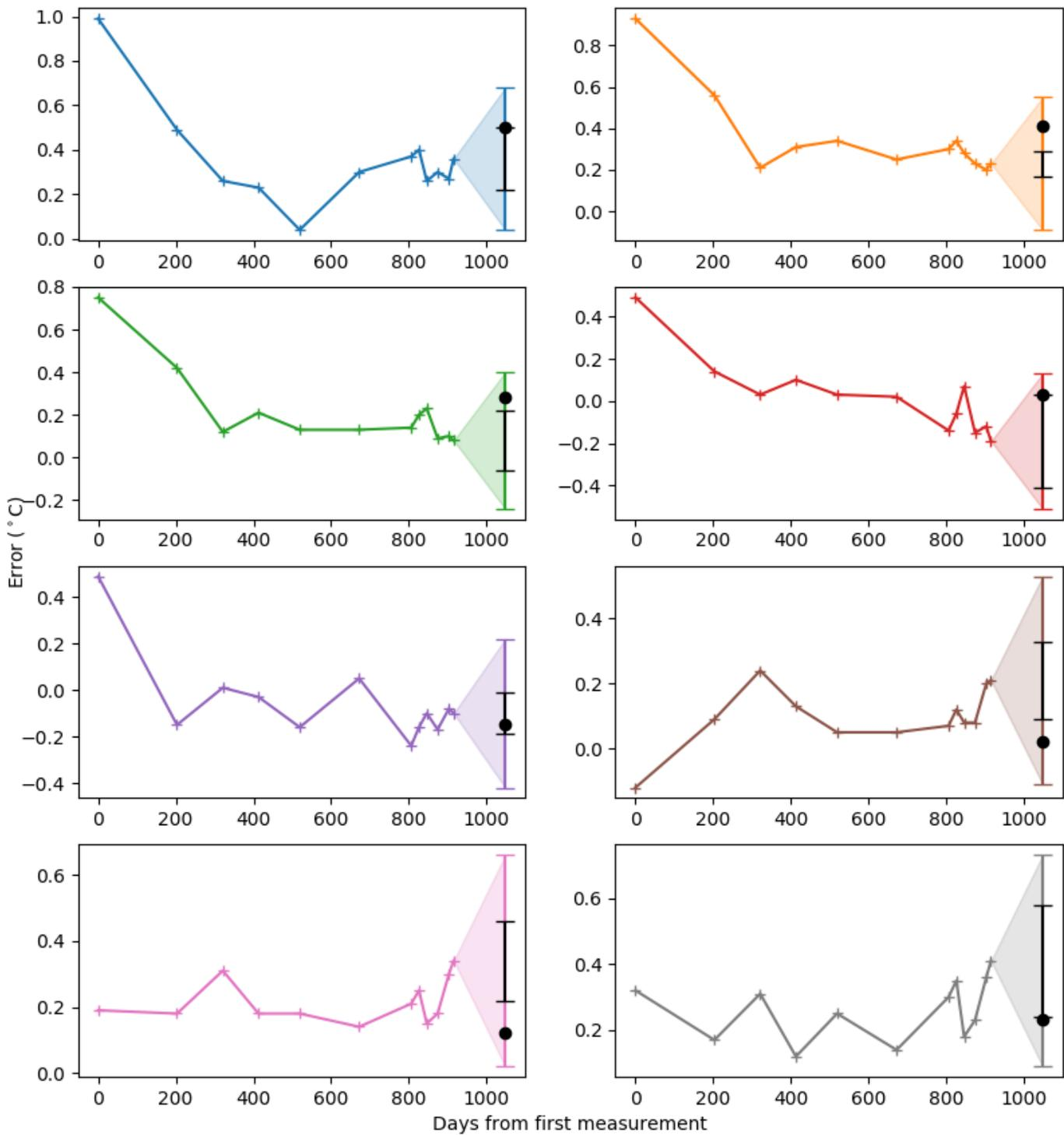
Fig. 5. Prediction of the interval in which the next calibration result will lie, calculated traditionally (black error bars) and using a new approach (coloured error bars), compared with actual measurements (black dots).
