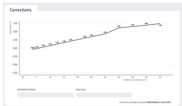
Fig. 4. Corrections calculator in LorisQ (IR thermometer)
