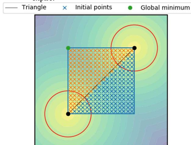
Fig. 3. The algorithm divides the room into triangles and in each calculates local optima (farthest points) from already determined control points. Subsequently, the farthest point is selected from this set of local optima and determined as the global minimum for the given iteration – the green point. At each iteration, a new background contour is calculated, which displays the distance from the control points in color.
