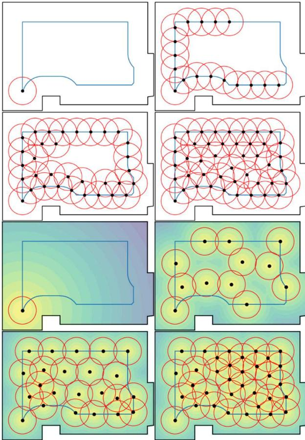
Fig. 5. The room is characterized by a more complex area where control points may occur. The results of the first algorithm are shown in the upper part. The figures show how the algorithm first determines the border control points in the marked area and then passes into the inner area of the room. The second algorithm created a network of control points, focusing on successively spaced control points throughout the area, as can be seen from the bottom figures.
