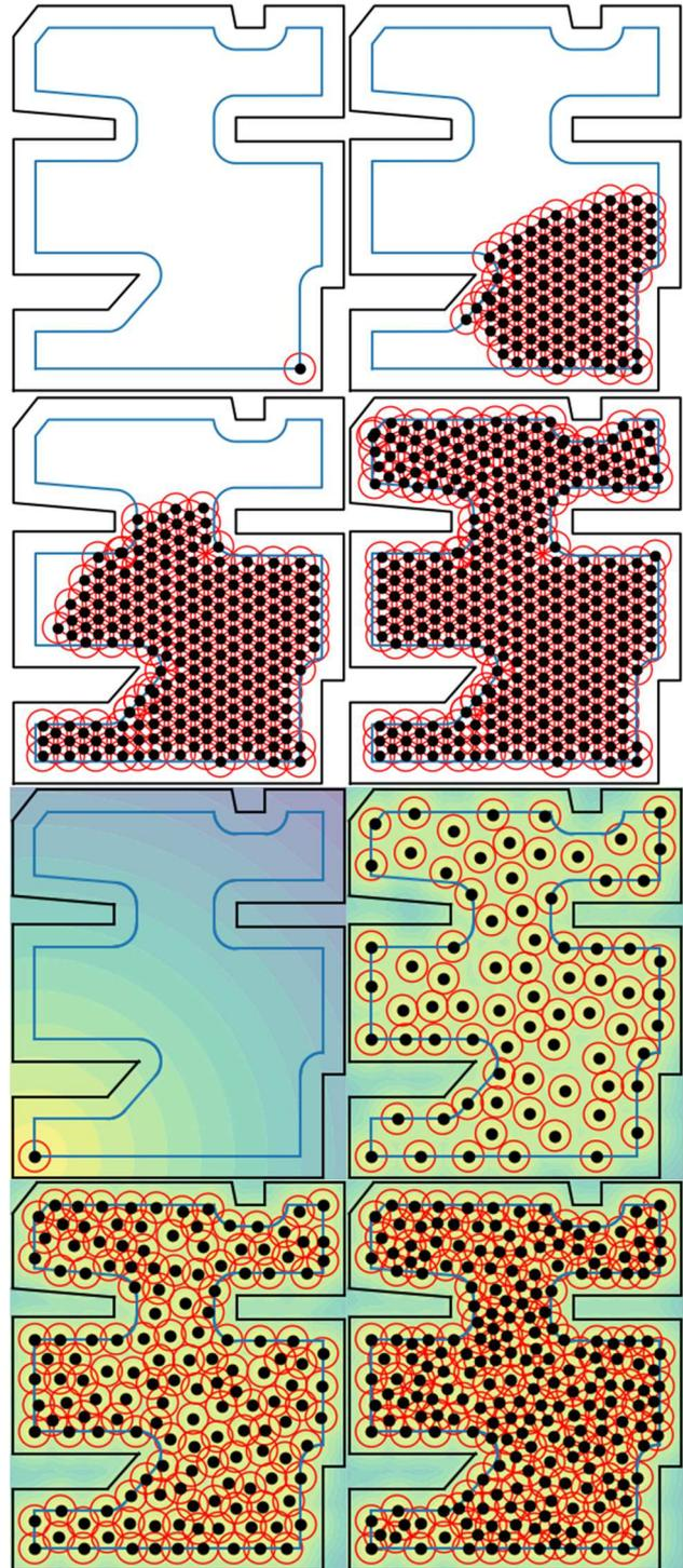
Fig. 6. To test both algorithms in demanding conditions, we created an intricately articulated and large room. Both algorithms proceeded as expected in determining the control points. The results show that the algorithm for long-term stationary noise determined significantly more control points than the algorithm for regular short-term noise.
