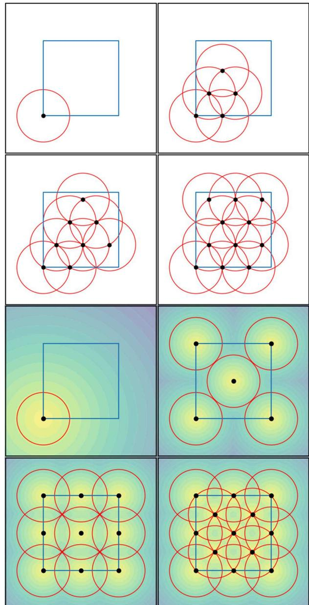
Fig. 4. The first top four images show the first algorithm that determines the control points for long-term stationary noise. The algorithm gradually adds control points where the intersection of the 0.7 m boundary with the other boundaries (red circles) occurs. An algorithm created the lower quartet of the image for regular short-term noise. The algorithm focuses on covering the area as much as possible in each iteration.
