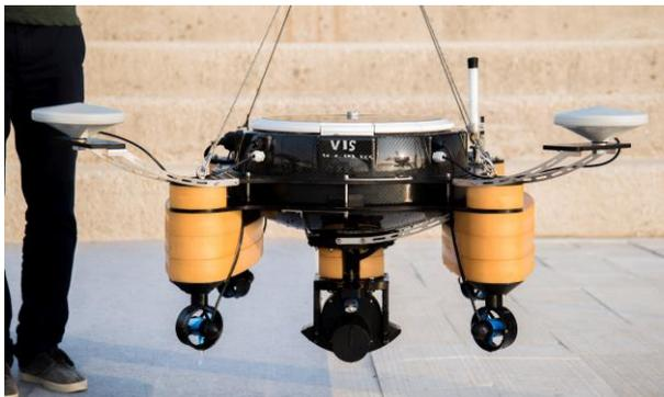
Fig. 1 System used for inspection. It consists of Acoustic Multibeam Sonar (in the middle below the vehicle) and Autonomous Surface Vehicle with its navigation, communication and propulsion payload.
