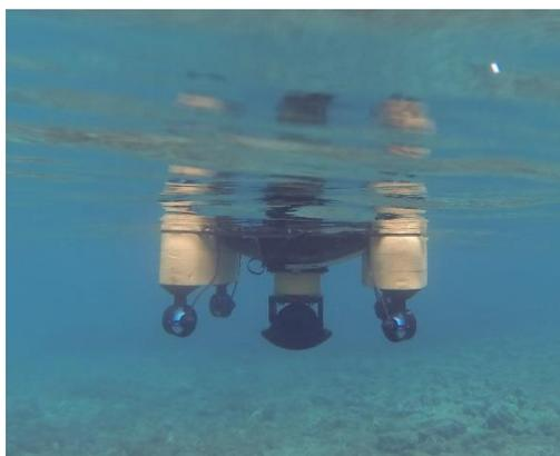
Fig. 2 The system in the water with sonar attached
