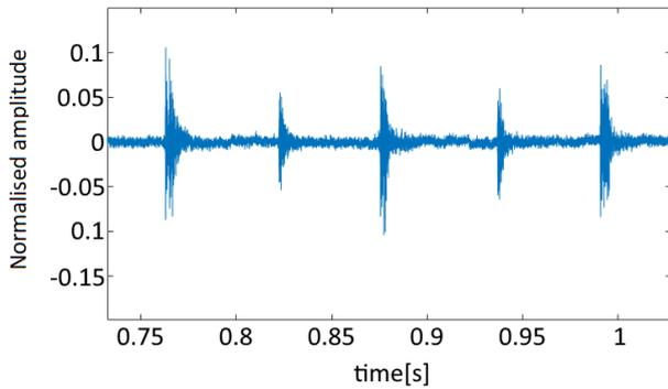
Fig. 5. Time-domain representation of the ratchet-generated pulse
