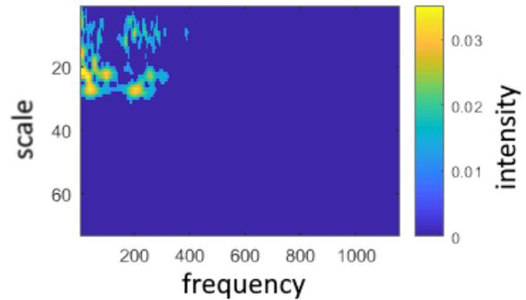
Fig. 6. Ratchet-generated pulse scalogram
