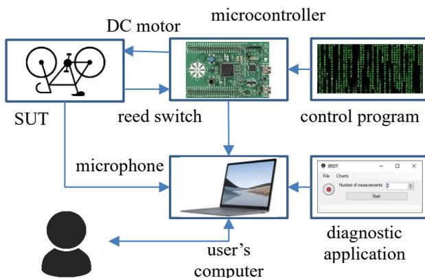
Fig. 3. Measurement system for the ratchet mechanism diagnostics
