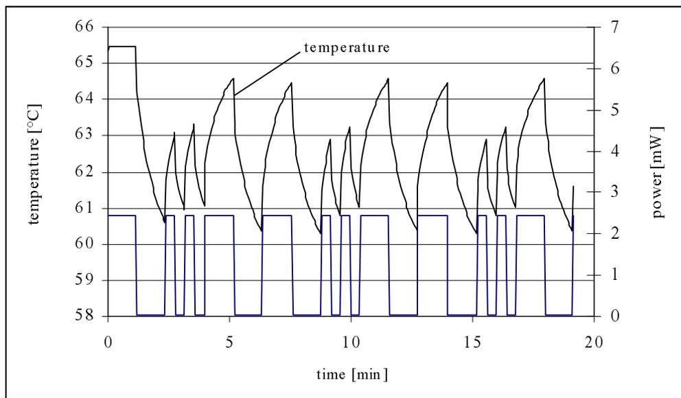
Fig. 2. The measuring data from 10 mm diameter thermometer during estimation of dynamic model with help of "in-situ" method and MBS 3311 signals using
