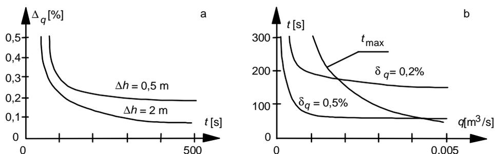
Fig. 1. Measurement possibilities of calibration system: a - error as a function of the time of filling the measuring tank, b - time of filling the measuring tank as a function of flow-rate
