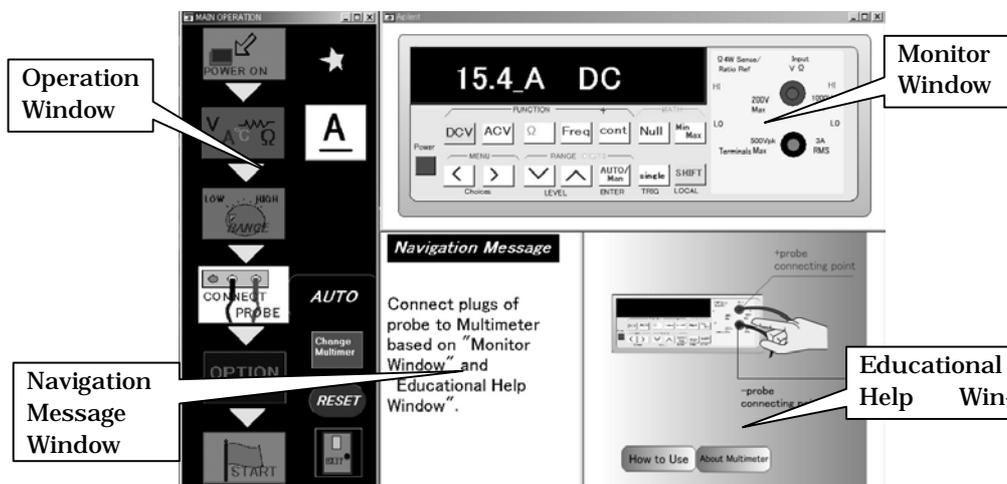
Fig.3. Initial screen of User Interface of multimeter
