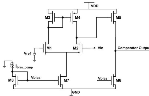
Figure 9. Schematic of the Comparator
