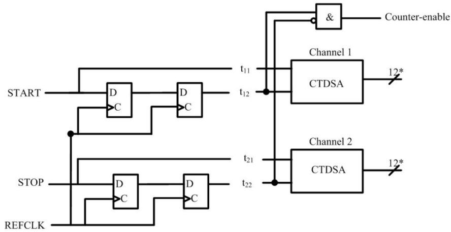
Figure 3. TDC with ns-level DR & sub-ps-level resolution
