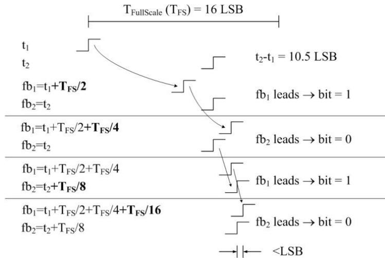
Figure 2. Operating principle of a 4-bit CTDSA method as a timing diagram [2].
