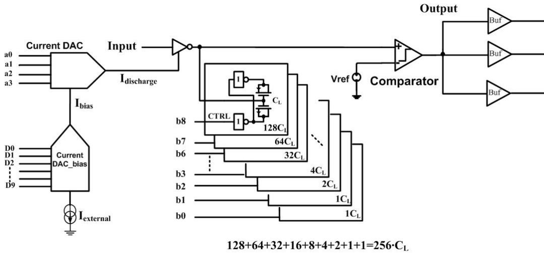
Figure 5. 12 bit Digital-to-time converter (DTC).
