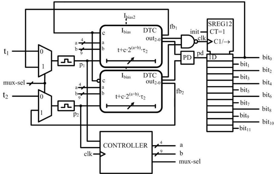
Figure 1. Block Diagram of CTDSA
