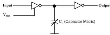
Figure 6. Previous Digital-to-time converter (DTC)
