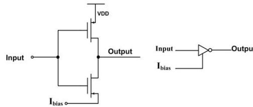
Figure 8. Schematic of Adjustable and Selectable Delay Cell
