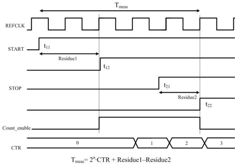
Figure 4. Operating principle of the TDC as a conceptual timing diagram.
